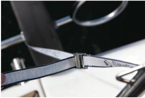
10. Fasten the straps with the buckle to the pushpit and adjust the height.
