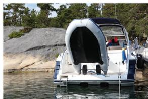
23. If used on top of a swim platform, the FLEX must be properly fixed.
