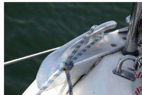
17. Fasten the ropes from the dinghy as far out on the sides of the boat as possible.
