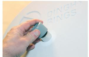
3. Attach the plastic end bushings to the pipe, press firmly by hand.
