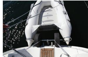
15. Raise the dinghy to standing position by pulling the ropes. Two ropes/straps needed.
