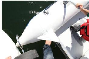
14. Take one pontoon end at a time and put into the rings. Use your foot or hand to guide.
