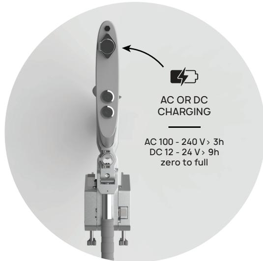
Integrated 1085 Wh battery is fully protected from all weather conditions and contains enough juice to get you more than 14 miles of range at a 3 mph cruising speed on a tender boat.
